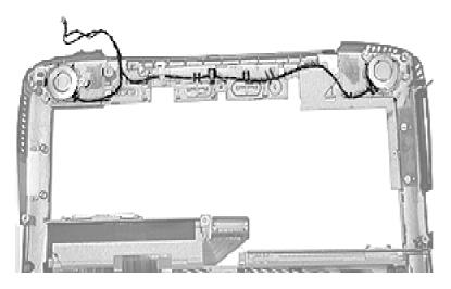
Release the speaker cable from its holding bracket.
