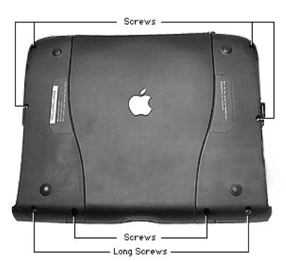
Turn the case over and remove the eight screws around the perimeter of the bottom case.
