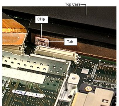
Find the metal locking clip located on the top case wall near the modem connector. Press on the tab with a flatblade nylon tool to release it from the metal clip.
