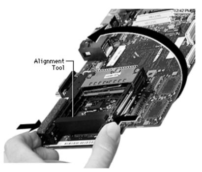
Pinch the ends of the cardcage together and turn the I/O logic board back over.
