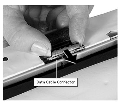
Use a nylon tool or pick to push the data cable connector on the side of the display to the right and gently pull the connector free.
