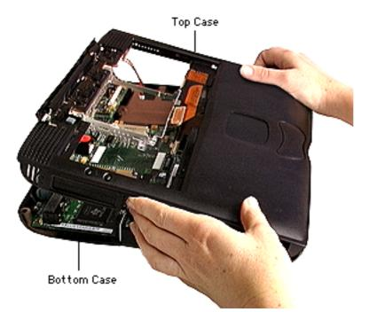
To Replacement Note: make sure the expansion bay flip door is aligned properly, push in on it when you replace the screw near the expansion bay flip door.
