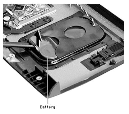
Lift the backup battery cable from its channeling.
