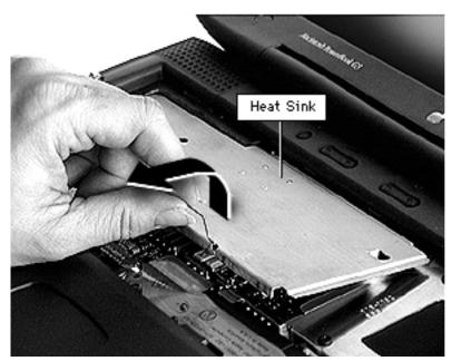
Lift up on the front handle and pull forward to clear the tabs from the slots at the back of the heat sink.
