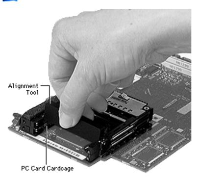
Turn the I/O logic board back over and insert the alignment tool between the inner sides of the PC Card cardcage.
