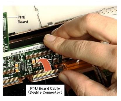
the PMU board to the slots in the case. Then connect the cables in reverse order.
