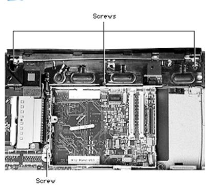
Remove the three screws under the clutch cover.
