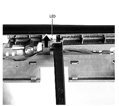
4 Carefully bow the LED out with the flat end of a nylon tool to release it from its holding tab and pull up on the cable.
