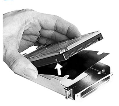
Remove the hard drive and hard drive insulator from the bracket.
