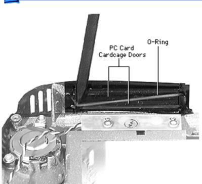
1 Remove the O-ring from its retaining hooks.
