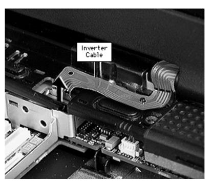
Use a nylon tool or other non-metal tool to unlock the inverter cable from the connector.
