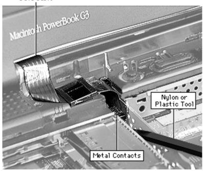
Warning: The cable connectors on the inverter cable and data cable have exposed metal contacts. Use only a non-metal tool to connect and disconnect these cables or you could short out the system.
