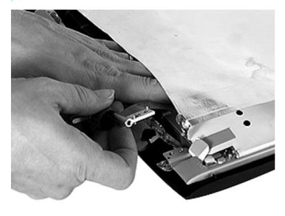
kapton tape holds the data cable in place. If it does, use the flat end of a nylon tool to loosen the tape.
