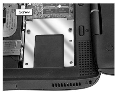
1 Loosen the screw holding the hard drive bracket.
