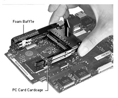
Turn the I/O logic board back over and pull up on the PC Card cardcage to release it from its double connectors.
