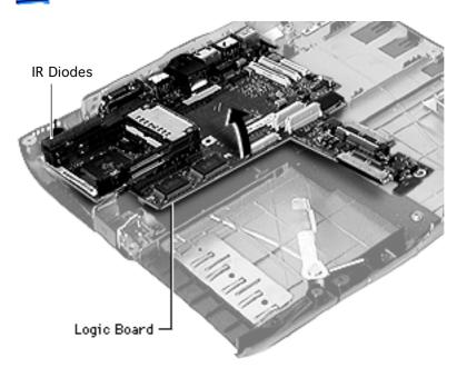
Hold the sides of the I/O logic board and lift up, then pull forward.
