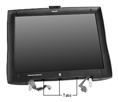
Insert the flat end of a nylon tool in the three tab openings at the bottom of the display and press down. Make sure the tabs on the bezel spring clear of the housing seam before proceeding to the next step.
