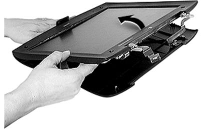
Tilt the display screen up and lift the bezel from the bottom to separate the two halves of the display.
