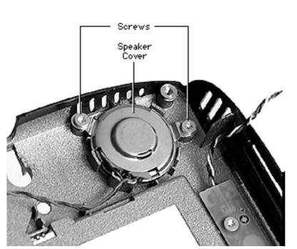
1 Unscrew the two screws on both the left and right speaker housings.
