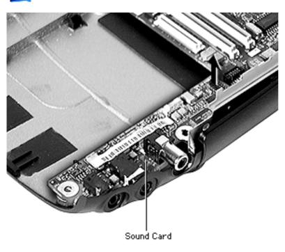
Gently press away on the case, then lift the sound card straight up.
