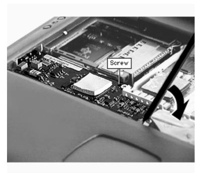
3 Lift up slightly and pull the modem to the right.
