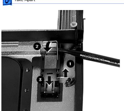
Lift up on the wire hook with a screwdriver and move it off the anchoring post.
