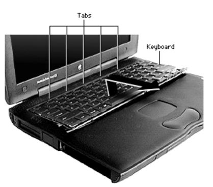
Lift the bottom portion of the keyboard up slightly and pull it back to disengage the five metal tabs holding the keyboard in place.
